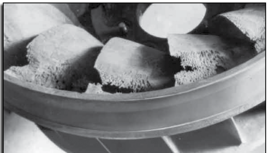
Figure 1: Pump damage from improper hydraulics. (Courtesy Caltech)
