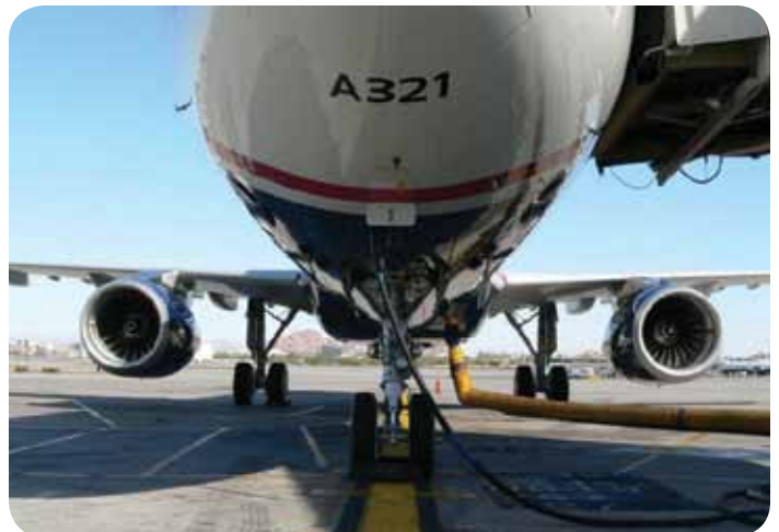
Ground power systems and preconditioned air units can help airlines reduce the need to fire aircraft auxiliary power units.
