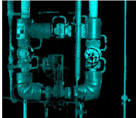
A point cloud created by laser scan data shows a rendering of an existing control valve station.
