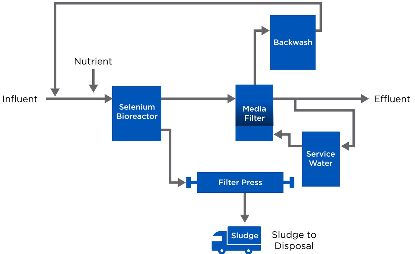
*Fluidized Bed Reactor Process Flow Diagram*
