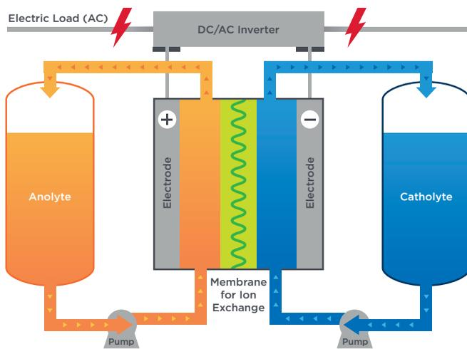
**FIGURE 1:** FIGURE 1: Diagram of flow battery process. Source: Summary of 2017 NASA Workshop on Assessment of Advanced Battery Technologies for Aerospace Applications.
