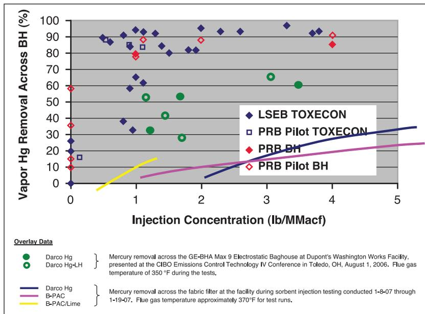
Figure 2. Overlay of facility's sorbent injection test results against other full-scale baghouse sorbent injection tests.
