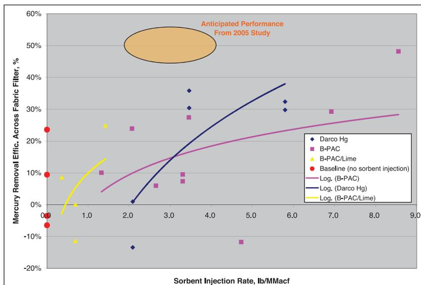
Figure 1. Mercury removal efficiency across the fabric filter vs. sorbent injection rate.
